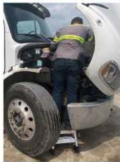
The 15LNCMINSTAND and 20LNCMINSTAND fit between the tire and bumper and provide stable slip-resistant platforms to work on the truck engine.
