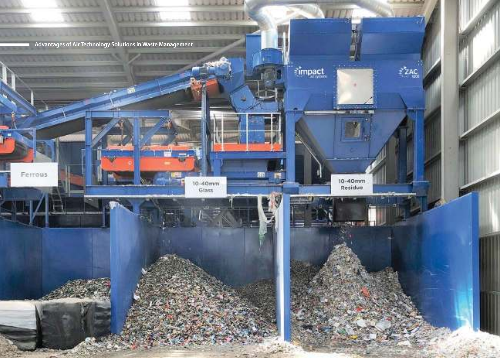
Glass clean-up system (Zigzag Air Classifier) in material recovery facility.
